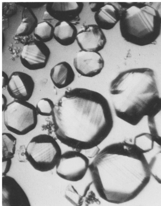
Fig. 3. CF-4 cubic-octahedral crystals under cross polarized light, \times 80 (grown in the MA–glycerine–SiO 2 –H 2 O system).
